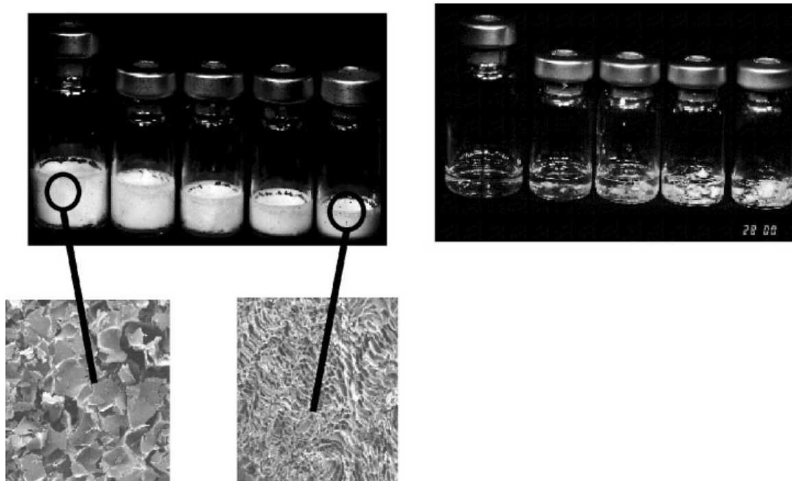
Figure 1. Lyophilization of a monoclonal antibody as a function of loading concentration. Upper left panel: Loading concentration from left to right was 40, 60, 80, 100, and 110 mg/mL, respectively, while maintaining the same total mass of MAb and excipients. Lower left panels: Scanning electron microscopy of lyophilized solid for the 40 and 110 mg/mL MAb loading concentrations. Right panel: 10 min after reconstitution of vials in upper left panel to 125 mg/mL with sterile water for injection.
